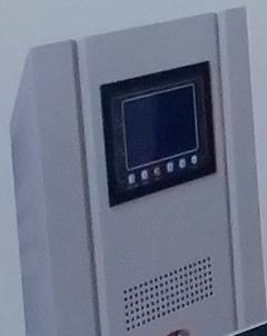
Our electronic voltage stabilisers offer the same general functionality as our electro-mechanical voltage stabilisers without the internal moving parts, eliminating the need for maintenance of the servo motor and variable transformer brush. The variable transformer and servo motor drive is replaced with an electronic voltage control system controlling the input. The transformer is designed to "buck or boost" the input voltage and so maintain the pre-set stabilised output voltage.
